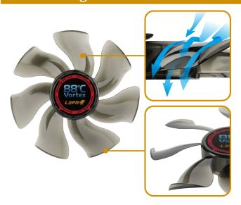
The S-blade composed with an advanced winglet structure which minimize the turbulence and stabilize the airflow; it allows the fan to operate with lower noise level and higher flow rate.
